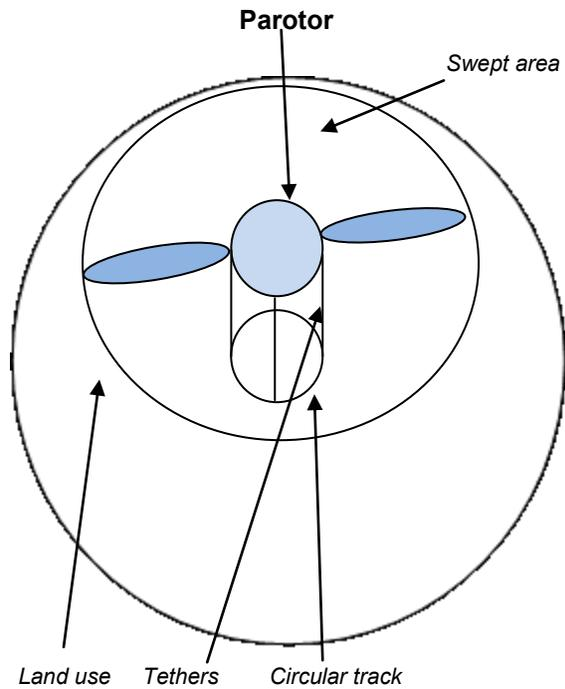
Figures 2a and 2b represent land area by view from the top. Both swept areas are considered as tilted (45°) areas planned on a horizontal plan.
